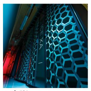
rank #31 540 nodes with: 2× Intel Xeon E5-2680 v4 4× NVIDIA Tesla P100 4× Intel Omni-Path
