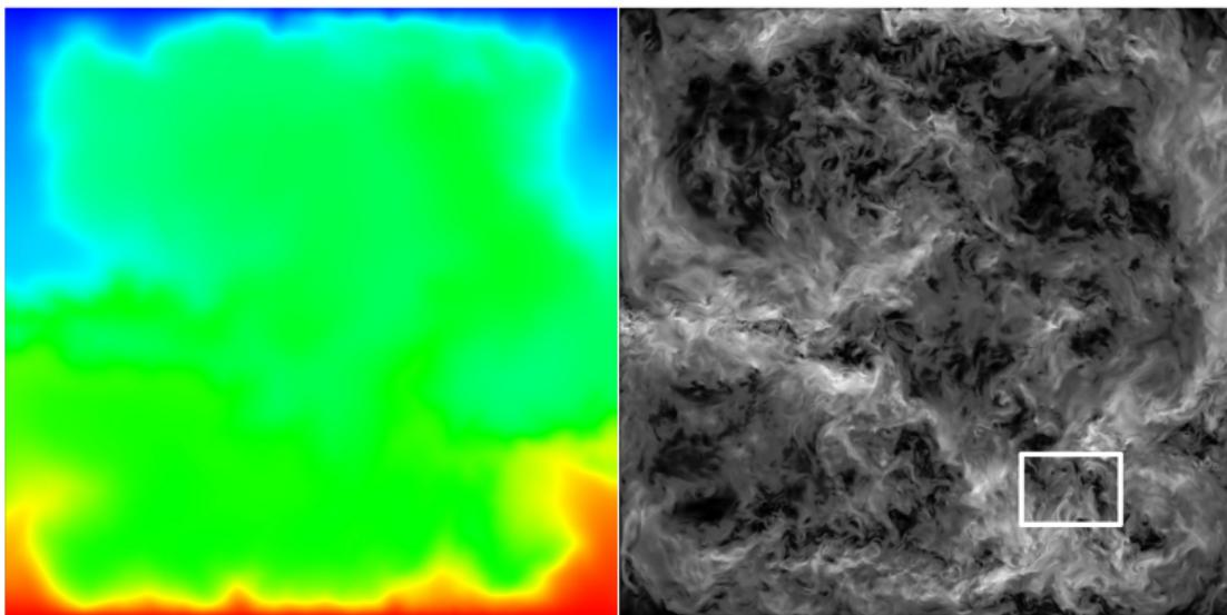
DNS of a RB at  $Ra = 7.14 \times 10^7$  and  $Pr = 0.005$  (liquid sodium)
