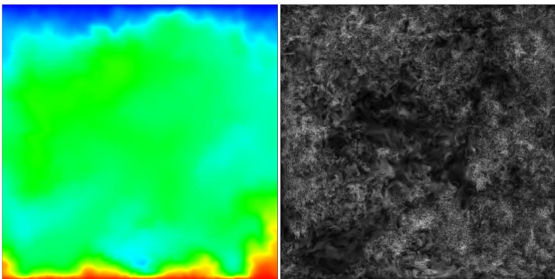
DNS of a RB at  $Ra = 7.14 \times 10^6$  and  $Pr = 0.005$  (liquid sodium)
