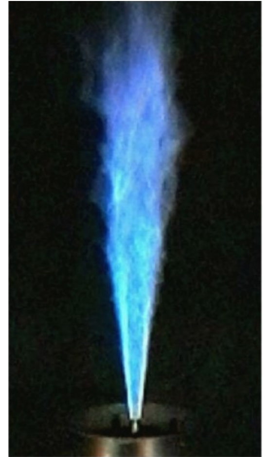
Fig.1 Hydrogen-methane jet flame example (source: DLR flame from TNF workshop)
