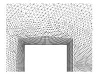
DNS<sup>3</sup> of the turbulent flow around a square cylinder at Re = 22000
